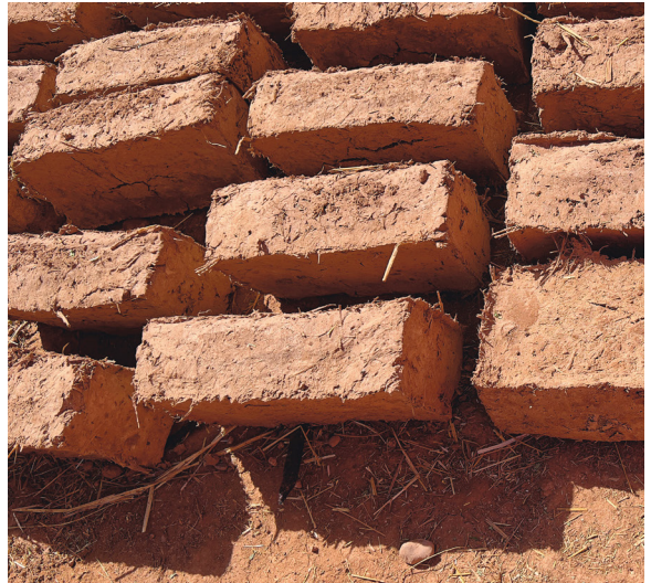
Earth and adobe (or compacted earth) or terracotta bricks form an alternative to concrete for individual housing. They account for half of houses worldwide.
